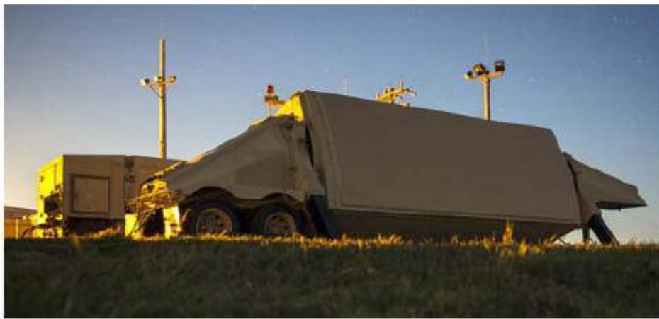
Figure 3 | The AN/TPY-2 is used to guard civilians and infrastructure in the U.S., deployed warfighters, allied nations, and security partners from ballistic-missile threats. Photo courtesy of Raytheon.
